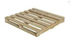
Light Medium (Transport) Dimension 1100mm X 1100mm X 140mm Weight Capacity 1000kg Top Boards – 7 (19mmX100mm X 1100mm) Bottom Boards - 3 (19mmX100mm X 1100mm) Bearers - 3 (27mmX100mm X 1100mm)
