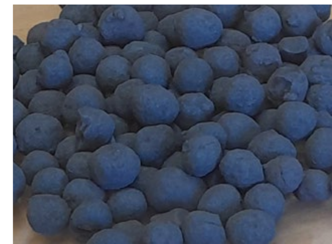
Direct Reduction (DR) pellet (small test) batch made from DR magnetite concentrate (<2 per cent Silica) produced from Duchess South Drill core using MEP2 technologies.
